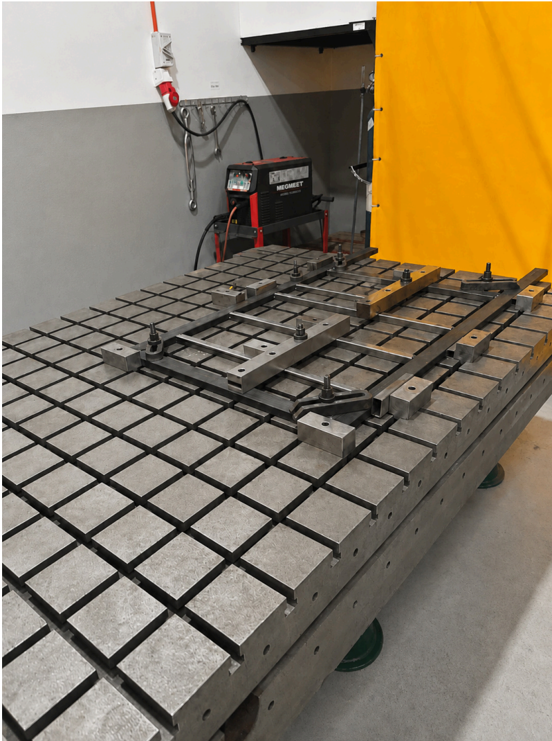
Actual KLH fit-up and fixture setup on a cast-iron grid table.
